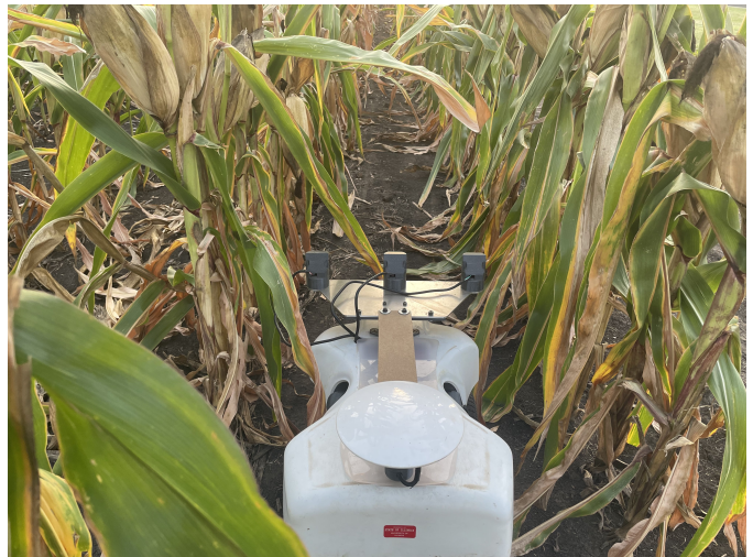
Fig. 1: Under-canopy navigation is challenging due to the tight space to traverse between the crop rows, frequent occlusion, and large variability in the appearance of the environment.
